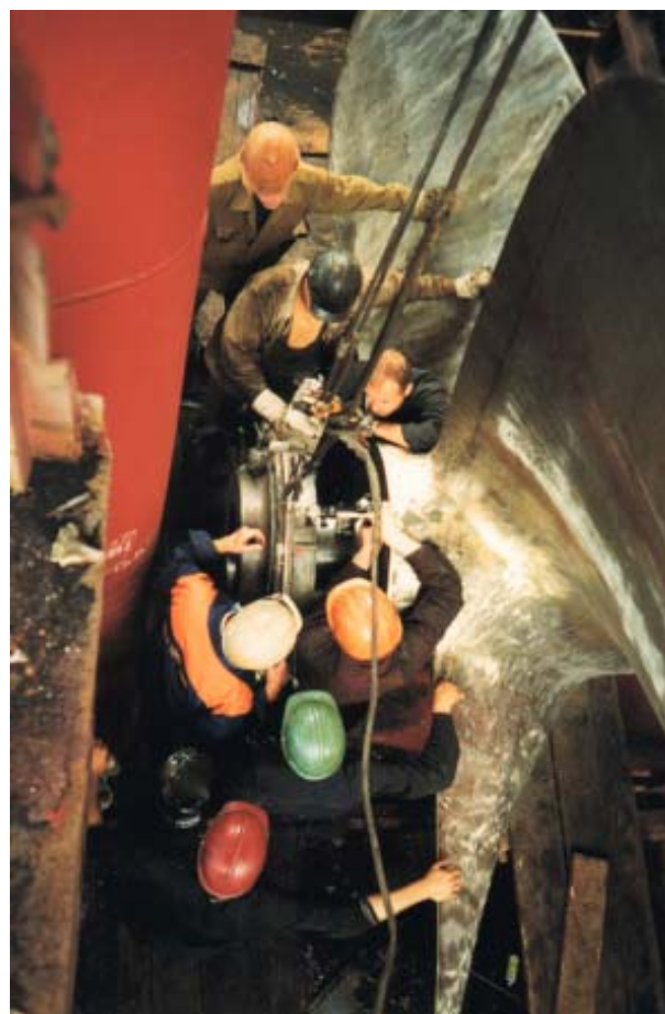
The correct way to replace a tailshaft nut
